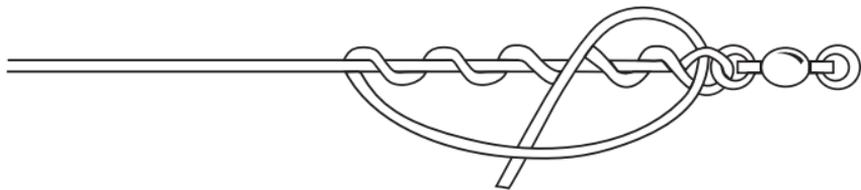
Hold the tag end of line while pulling up the coils. Make sure the coils are in a spiral, not lapping over each other. Slide tight against the eye. Clip the tag end.
