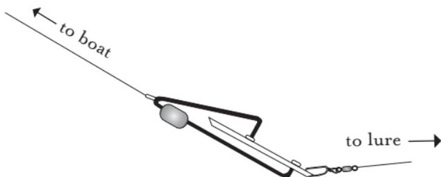
In these instances, it is helpful to be able to reset the planer without reeling it all the way to the boat. Pull in several feet of line and then quickly release it. This slack in the planer line will allow the weight on the planer wire to cause the planer to nose dive and reset itself. If this doesn't work after an attempt or two, slow the boat speed and repeat the procedure. Again, this same procedure can be used if the planer should hit bottom and trip.
